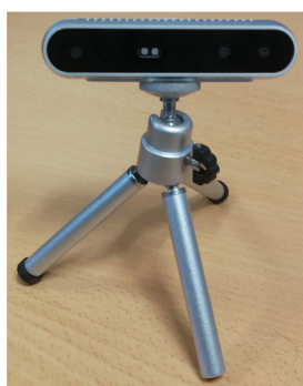
FIGURE 28. Intel RealSense D415 used for experiments, mounted on a tripod. The camera consists of a pair of depth sensors, an infrared projector, and an RGB sensor. The D415 model has a rolling shutter.
