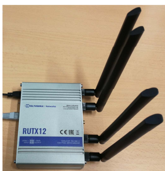
FIGURE 26. Teltonika RUTX12 used for experiment with the VPN 4G modem over CERN GPN connection type experiments.
