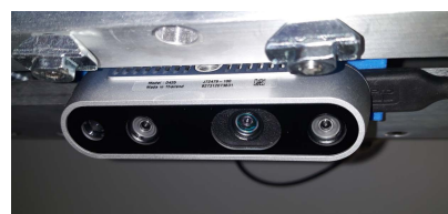
FIGURE 29. Intel RealSense D435, also used in the experiments, installed in the train inspection monorail wagon. The D435 model, compared to D415, has a wider field of view (FOV) and a global shutter.
