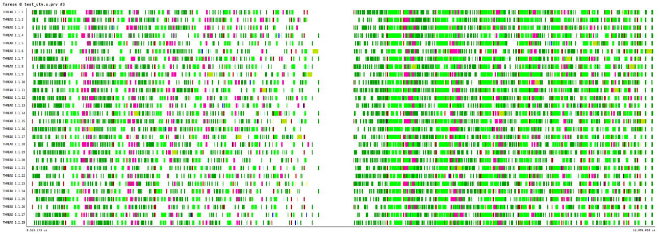
Figure 15: Execution traces for the algorithm-by-block of randUTV with n = 1920 and b = 384 in marbore (28 threads), without and with computation of orthonormal matrices (left and right parts of the trace, respectively).
