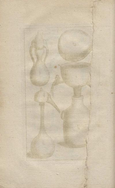
B. Its Head or Limbick with a nofe or fpont; having a narrowed neck fit for its Bolts-head Matrafs and well luted, to receive the volatile Spirits, Salts, which afcend.
