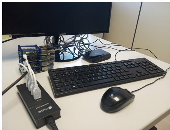
Figure 2: A Raspberry Pi cluster assembled during the course. Note that the 3D-printed structure that holds the Raspberry Pi devices is only used for aesthetics purposes.
