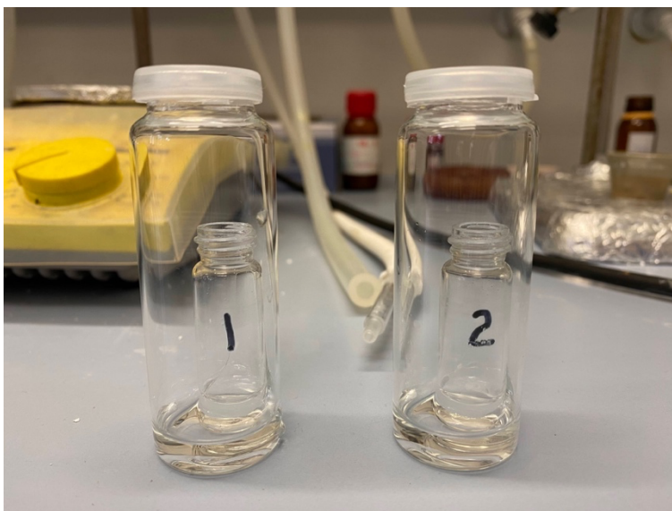
Figure 21. Procedure to determine if (\text{PyrSucVal})_2\text{Oct} forms a gel in water by smooth pH change. The vial with 2 mg of (\text{PyrSucVal})_2\text{Oct} dissolved in 1 mL HCl 0.1M is introduced in a closed system containing concentrated aqueous \text{NH}_3 25%.
