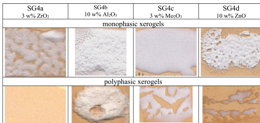
Fig. 15 Doctor Blade depositions of the monophasic and polyphasic xerogels fired with a single fire cycle.
