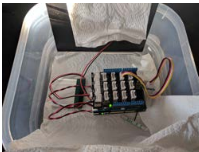
Fig. 5: A fully assembled experiment's IoT node
