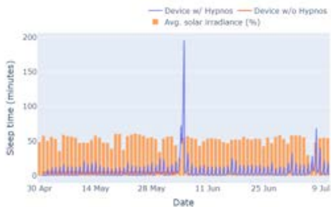
Fig. 10: The sleep times of the two IoT nodes, along with the average daily solar irradiance percentage
