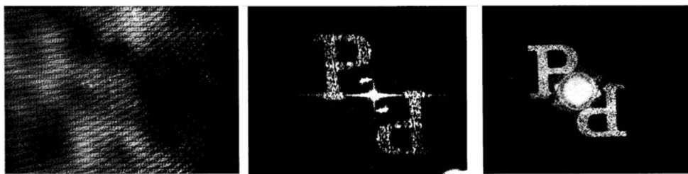
Fig. 1. (a) Detected hologram, (b) Computed image, (c) Optically obtained image. Reproduced from J. W. Goodman and R. Lawrence, “Digital image formation from electronically detected holograms,” Appl. Phys. Lett. 11 , 77–79 (1967), with the permission of AIP Publishing.
