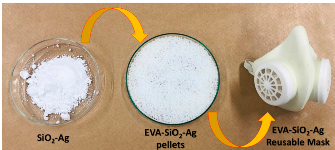
Figure 8. Reusable mask manufactured using the EVA-SiO 2 -Ag composite (Assis et al. [116]).
