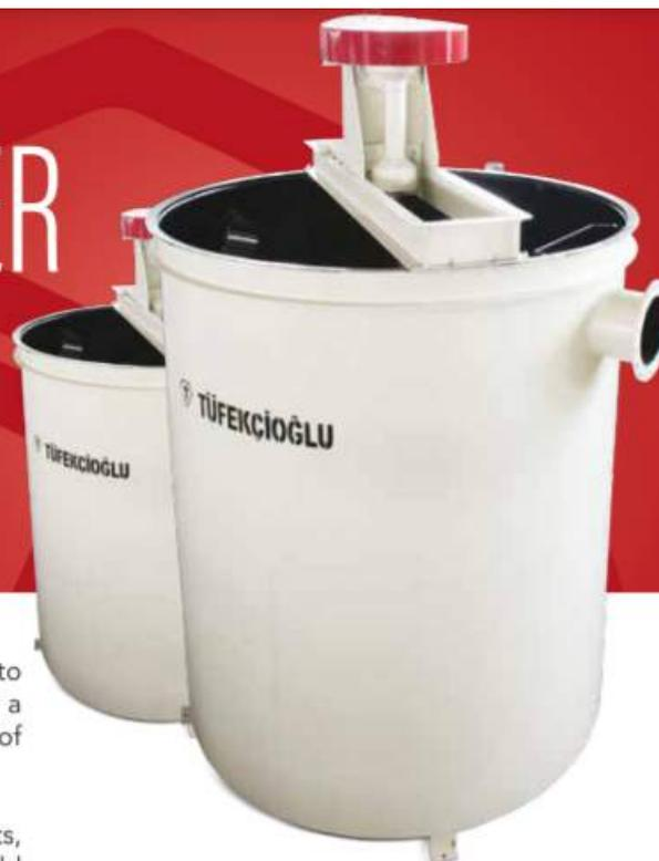
These tanks are designed and produced to condition pulps with flotation chemicals for a certain period of time for the preparation of minerals prior to flotation or depression.
