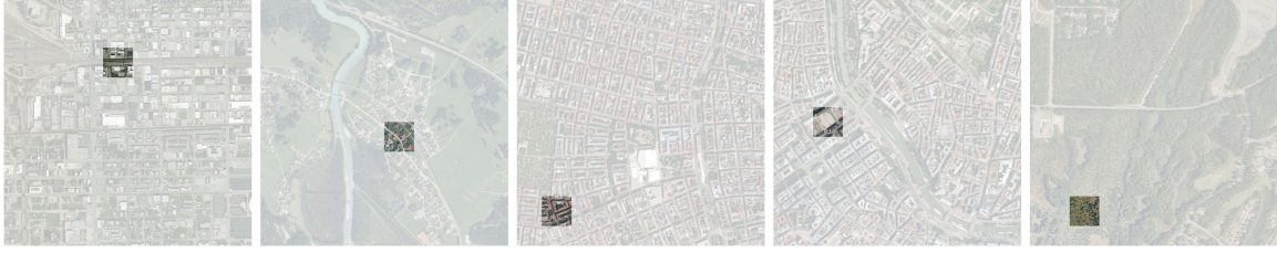
Fig. 3. Training set construction for the Inria dataset. For each tile of 2.25-km 2 area, we only randomly crop 0.0324-km 2 area with the spatial size of 600 × 600 pixels to be labeled. The others are regarded as unlabeled images in the training set.
