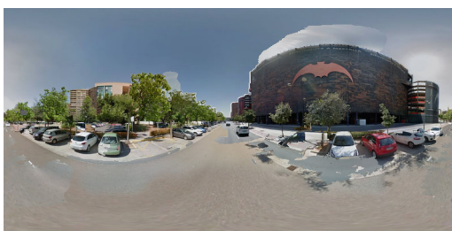
Fig. 12 Result of merging two panoramas without user adjustment where artifacts are clearly noticeable
