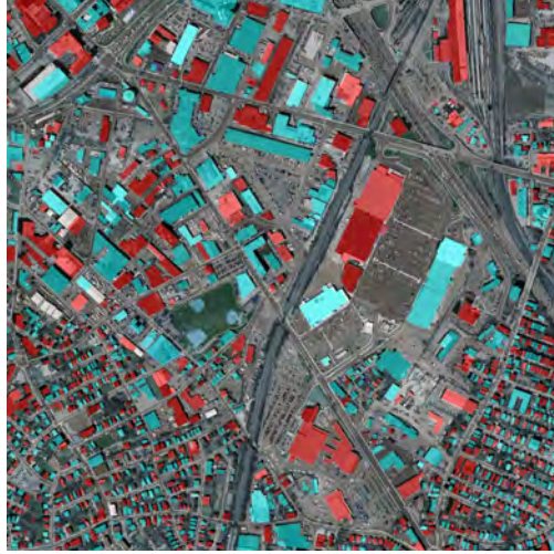
Fig. 1. An illustration of a satellite image containing buildings with missing annotations, where the cyan color denotes the available ground-truth footprints and the red color indicates the missing footprints.
