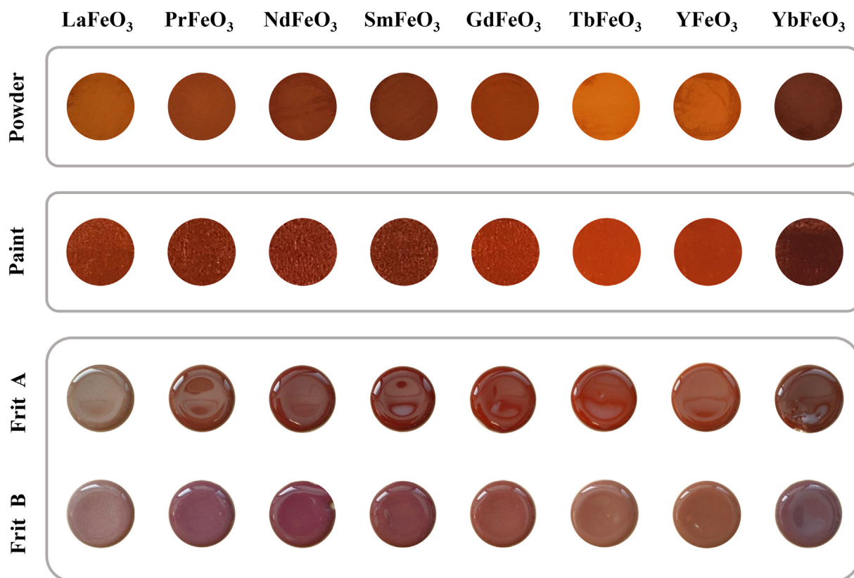
Fig. 9. Photographs of the powders, the pigment–siloxane paint mixtures and the pigments with glazes (frit A and frit B).
