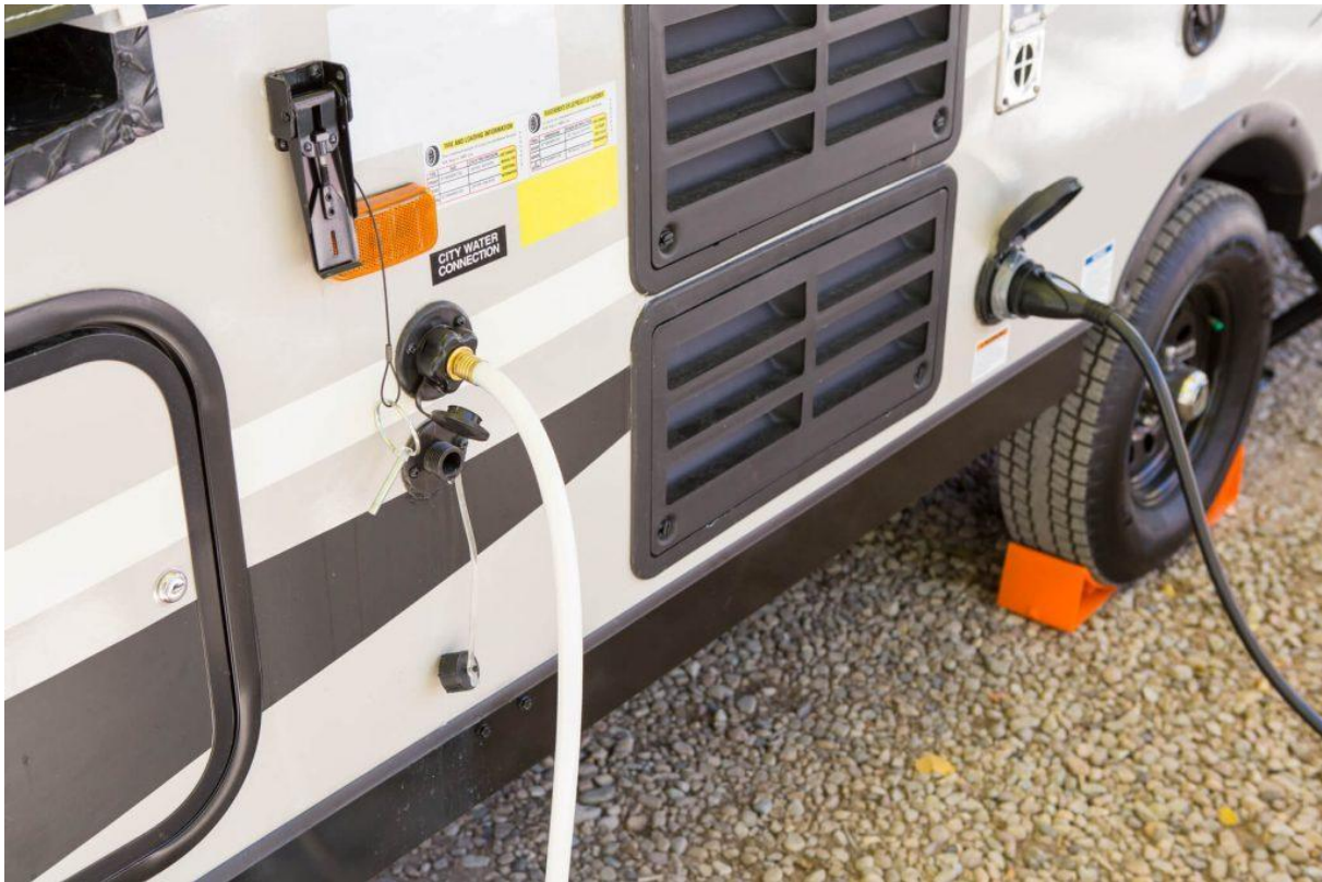
Figure 6. Light and Water Intake
