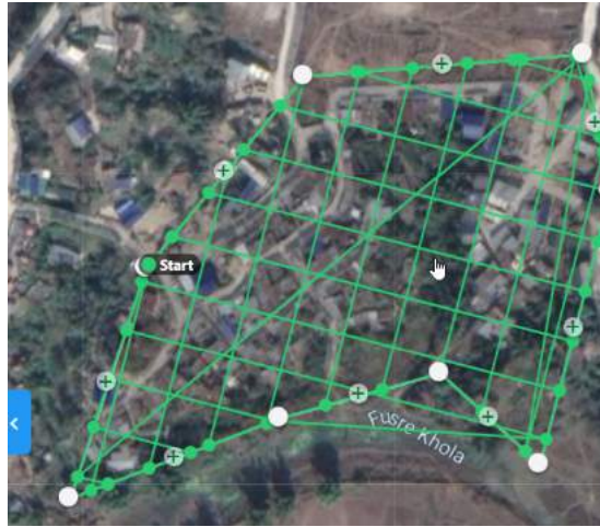
Figure 4.2: Flight planning for UAV using DroneDeploy. Green lines represent flight path for the user-specified configuration
