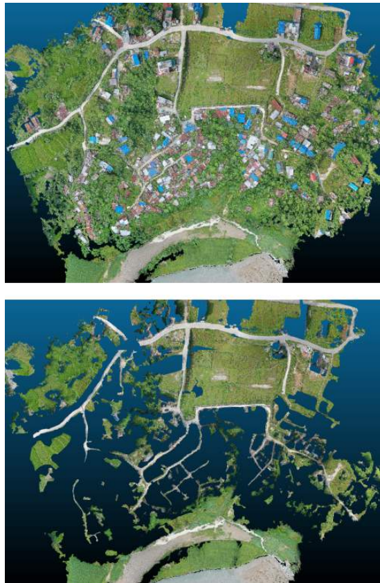
Figure A.1: Sample Point cloud before and after filtering. Top: Original Point Cloud, Bottom: Filtered point cloud
