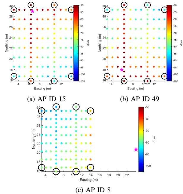
Fig. 2: Mean RSS values per reference point and device reference positions of three APs (Library, 5<sup>th</sup> floor). The device position is indicated with a star. Circles highlight the reference points whose values were used to train regression models.
