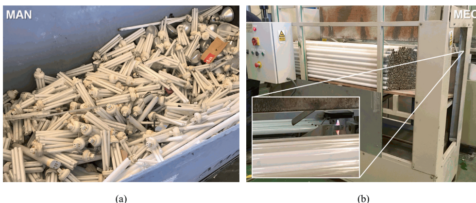
Fig. 2. The original spent fluorescent lamps: a) Manually processed; b) Mechanically processed.
