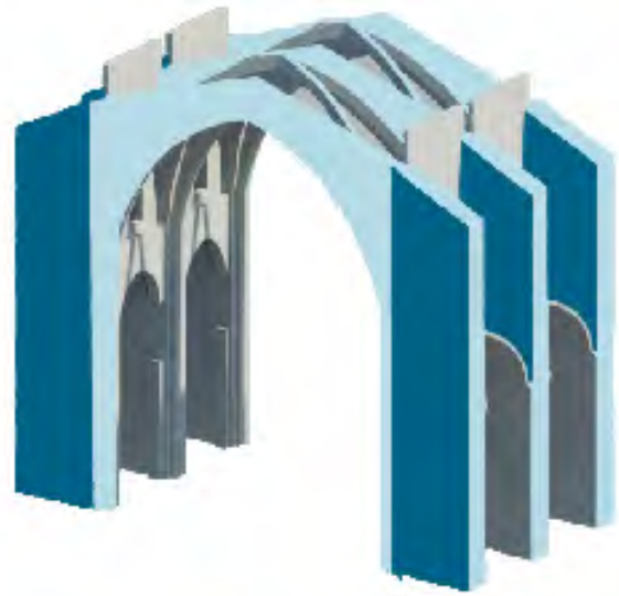
Figure 2. Structural plot of the Santos Juanes Royal Parish Church in Valencia, Spain.
