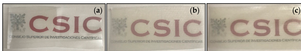
Figure 3. Visual aspect of: (a) YPACK210 film; (b) active multilayer films with cellulose nanocrystal (CNC) coating; (c) active multilayer films without CNC coating. Films are 5 cm × 2 cm.
