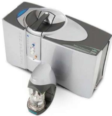
The Hydro EV has a unique dip-in centrifugal pump and stirrer design that achieves full and rapid dispersion in standard laboratory beakers, allowing close matching of the dispersant volume to the application requirements. Following measurement, the dispersion head can be raised out of the beaker, enabling quick cleaning and sample recovery.
