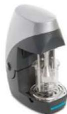
**Hydro EV** - A unique dip-in, semi-automated wet sample dispersion unit that can be used with 250mL, 600mL and 1000mL standard laboratory beakers.
