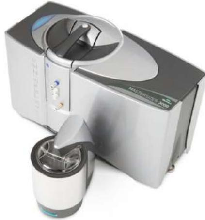
Intended for applications where sample availability is not an issue, the Hydro LV is ideal for measuring larger particles and broad size distributions, which demand larger sample volumes to ensure representative measurement.
