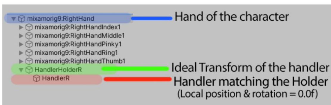
Figure18. Handler and holder of the new connector restructured in hierarchy.
