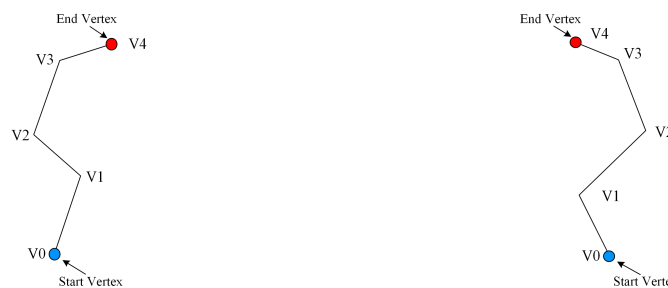
(a) The CD for this road is (r, l, r, r). (b) The CD for this road is (l, r, l, l).
