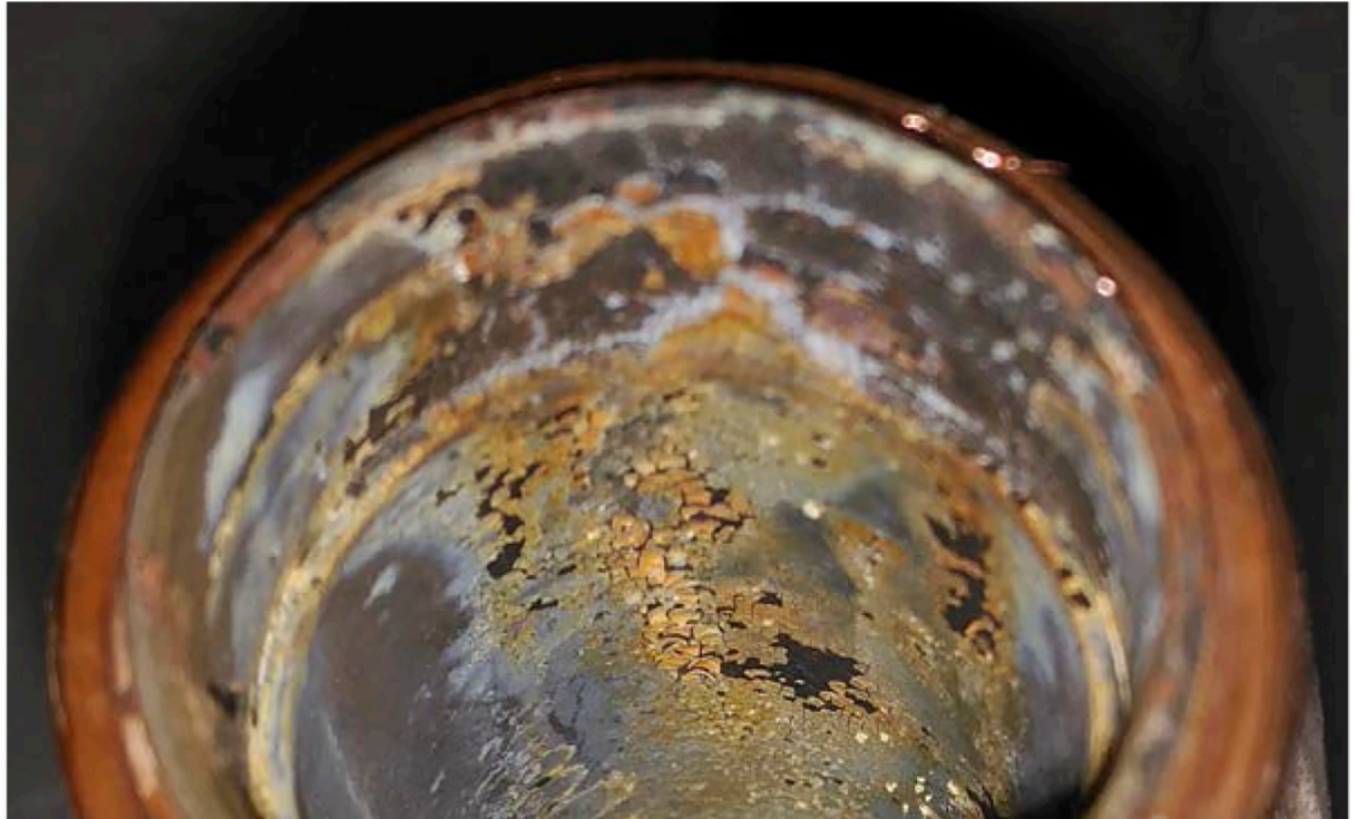
Fig 7. Nanoparticle deposition after the efficiency tests.
