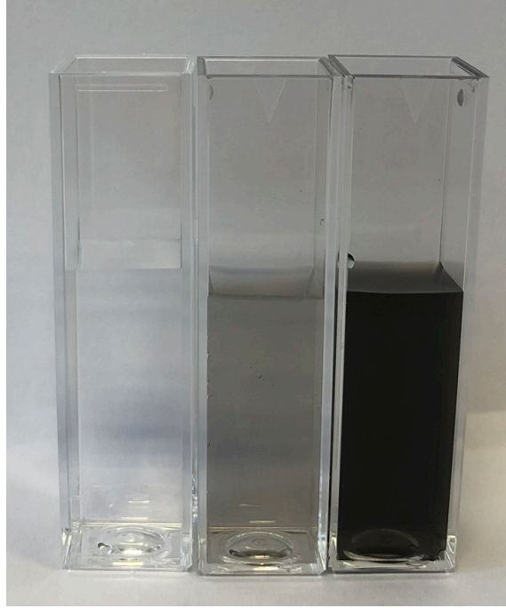
Figure 1 Samples of the base fluid and water-based carbon nanofluids with different concentrations.
