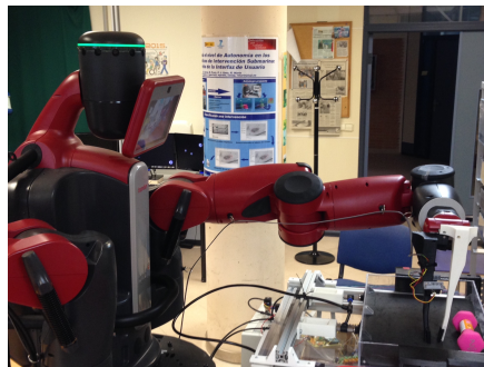
FIGURE 5.1: The distance to the bin results in many unreachable configurations
