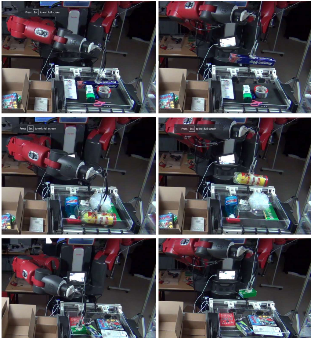
FIGURE 4.9: CNA with vacuum successful grasp of the reynold's wrap, tennis ball container and irish spring soap
