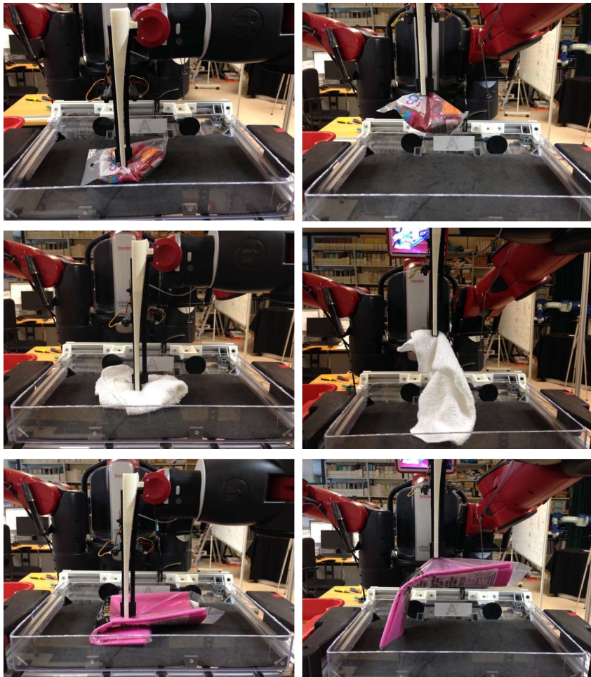
FIGURE 4.10: CNA with Pincher successful grasp of balloons, face cloth, and table cloth
