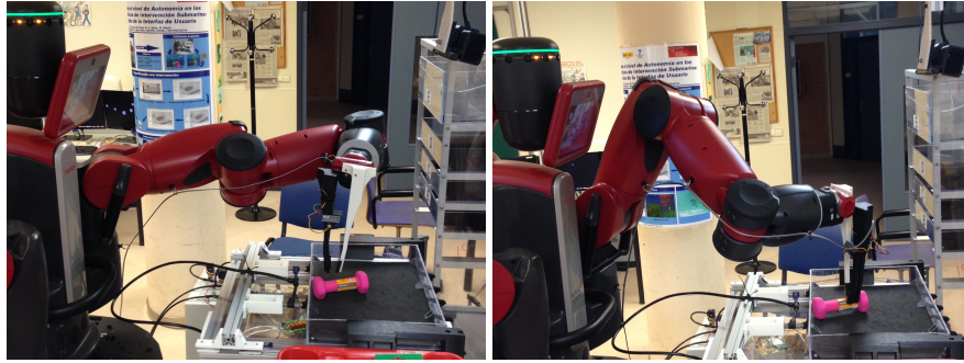
FIGURE 5.2: (left) Maximum angle restriction. (right) Constitutes a collision due to shoulder motion.
