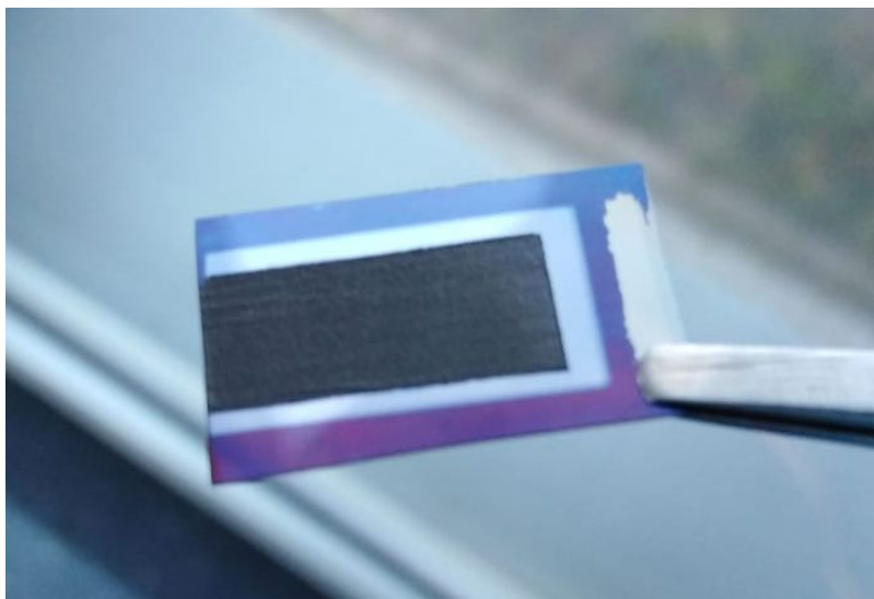
Figure S4. Picture of a p-i-n perovskite solar cell with the Cr/C back contact electrode, deposited on a flexible substrate.
