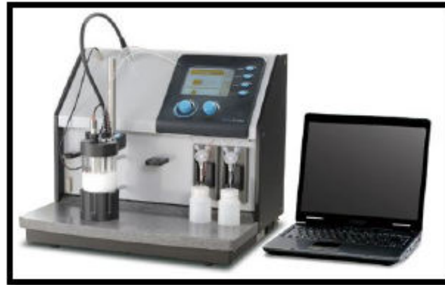
Figure 3 The Zeta probe used to measure Zeta potential of drilling fluids
