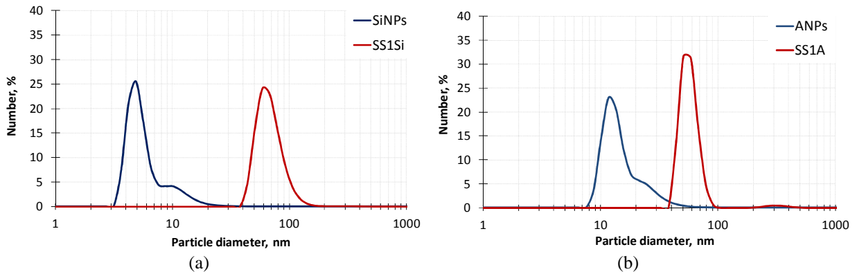
Fig. 1: Nanoparticle size distribution of the raw NPs dispersions \text{SiO}_2 NPs (a) and \text{Al}_2\text{O}_3 NPs (b) and the samples SS1Si (a) and SS1A (b).
