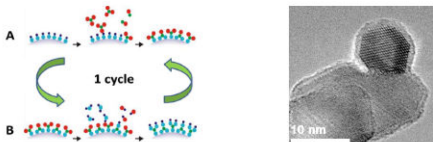
Figure 1. (left) Reaction mechanism of one cycle of atomic layer deposition. (right) Titanium oxide nanoparticles coated with aluminium oxide using ALD [3].
