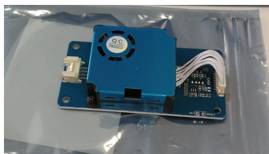
Figure 2. HM-3301 PM sensor.
