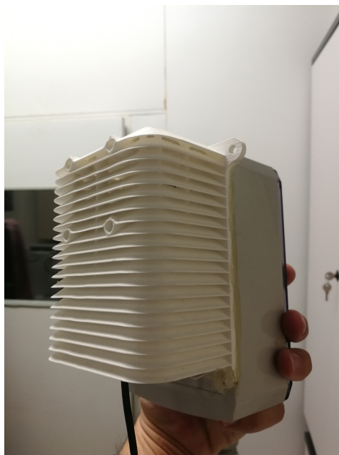
Figure 1. The 3D printed enclosure of the particulate matter (PM) sensor.
