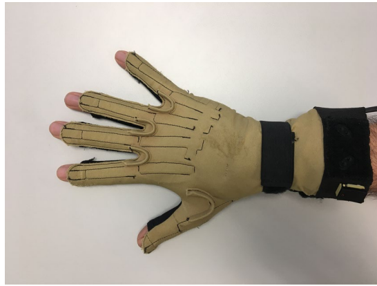
Fig. 1 Cyberglove I device and the strap used for the wrist sensors.
