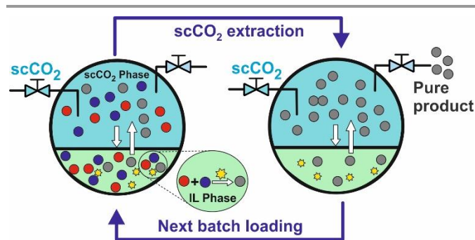
Fig. 3. General scheme for integrated reaction separation processes in IL/scCO 2 biphasic systems.
