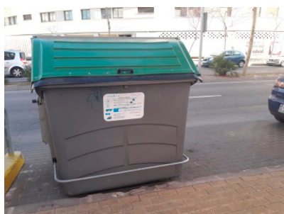
(c) Mixed surface bins (2.4 and 3 m 3 ). Automatic sideloading.
