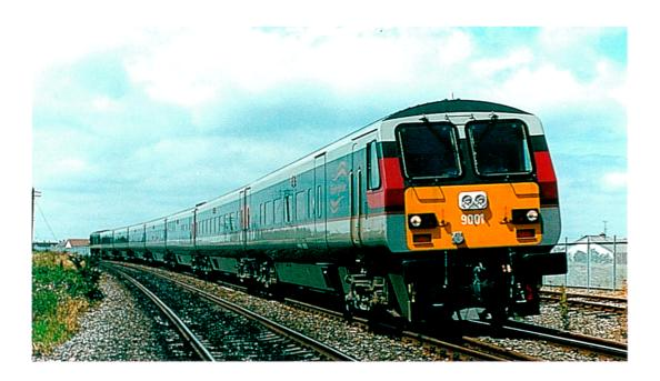
To achieve this, the control and signalling systems have been entirely modernised, level crossings automated and old-fashioned jointed track on wooden sleepers replaced by continuous welded track on concrete sleepers. Bridges and fences have been upgraded and new rolling stock introduced.
