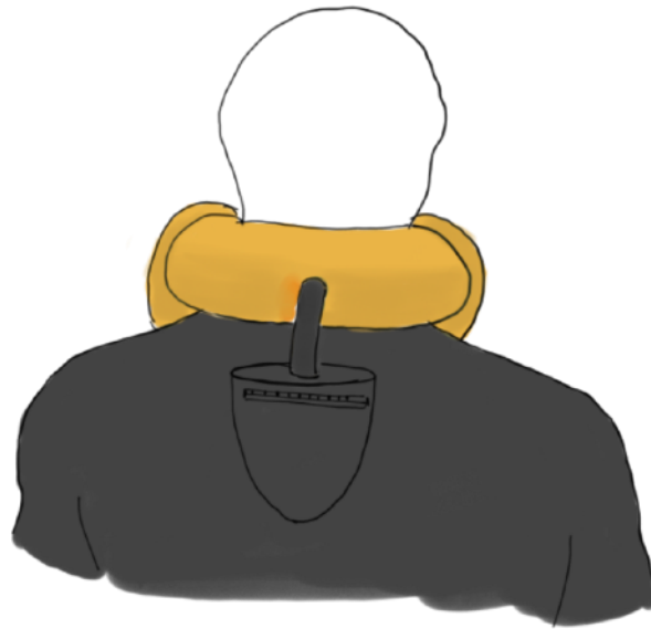
Sketch 1.8.2.3- connection between float and valve
