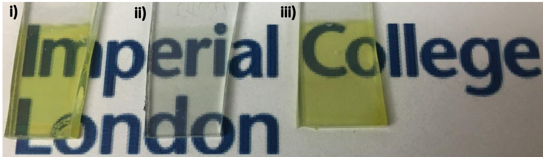
Fig. S3 UV-Vis spectra of photoanode films measured using a Shimadzu UV-2700 equipped with an integrated sphere. (a) Absorbance of films taking into account of transmittance, diffuse reflectance and specular reflectance. (b) UV-Vis spectra of bare BiVO 4 and WO 3 /BiVO 4 with varying thicknesses of BiVO 4 . (c) images of the films: (i) BiVO 4 , (ii) WO 3 and (iii) WO 3 /BiVO 4
