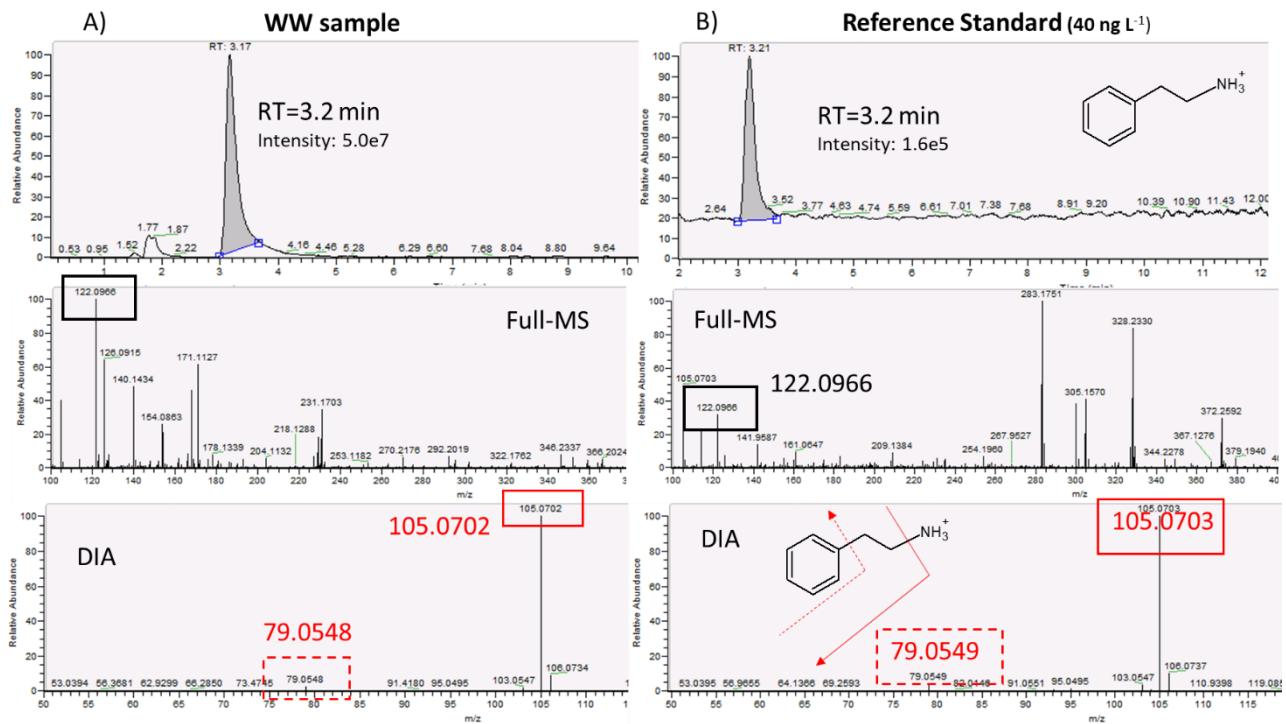
**Fig S3.** Chromatograms and MS<sup>2</sup> spectra for para-methoxyamphetamine (PMA) in A) wastewater and B) reference standard. Identification at confidence level 1.
