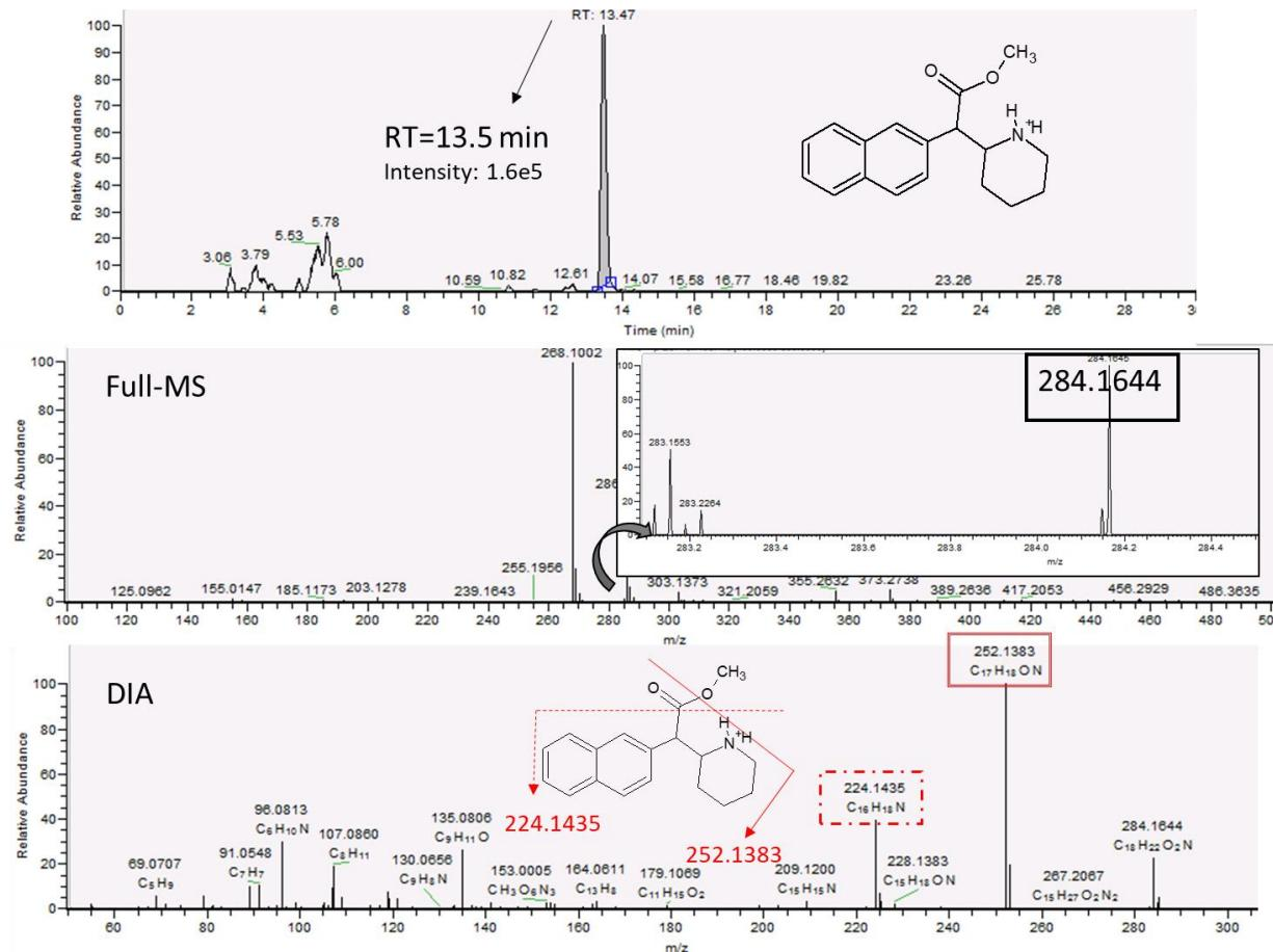
**Fig. S7.** Chromatogram and MS<sup>2</sup> spectra for the Isopropylphenidate in wastewater. Identification at confidence level 3.
