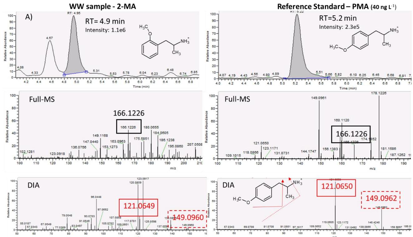
**Fig. S5.** Chromatogram and MS<sup>2</sup> spectra for the DOiP in wastewater. Identification at confidence level 3.
