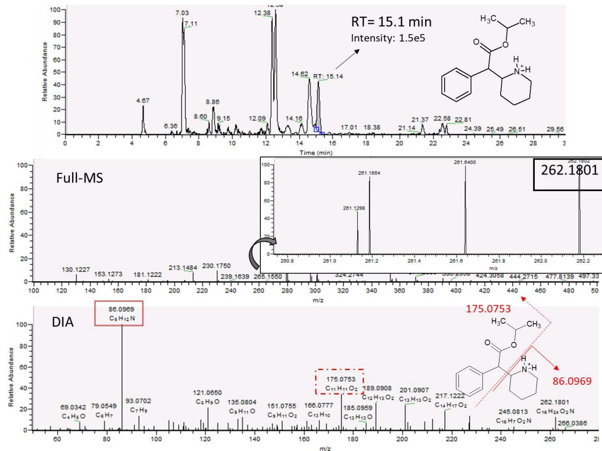
**Fig. S8.** Chromatogram and MS<sup>2</sup> spectra for the diphenidine in wastewater. Identification at confidence level 3.
