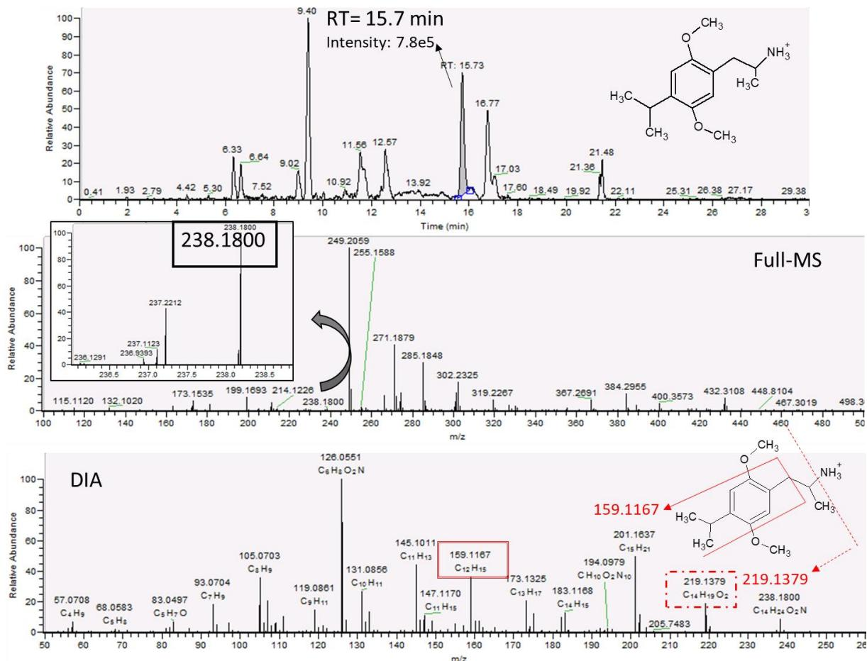
**Fig. S6.** Chromatogram and MS<sup>2</sup> spectra for the HDMP-28 in wastewater. Identification at confidence level 3.
