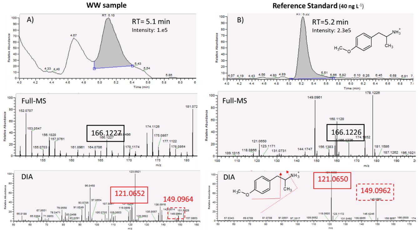
**Fig S4.** Chromatograms and MS<sup>2</sup> spectra for (A) 2-methoxyamphetamine (2-MA) in wastewater and B) analytical standard of *para*-methoxyamphetamine (PMA). Identification at confidence level 2.
