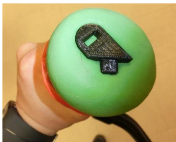
Illustration 9. Universal gripper grasping PART
