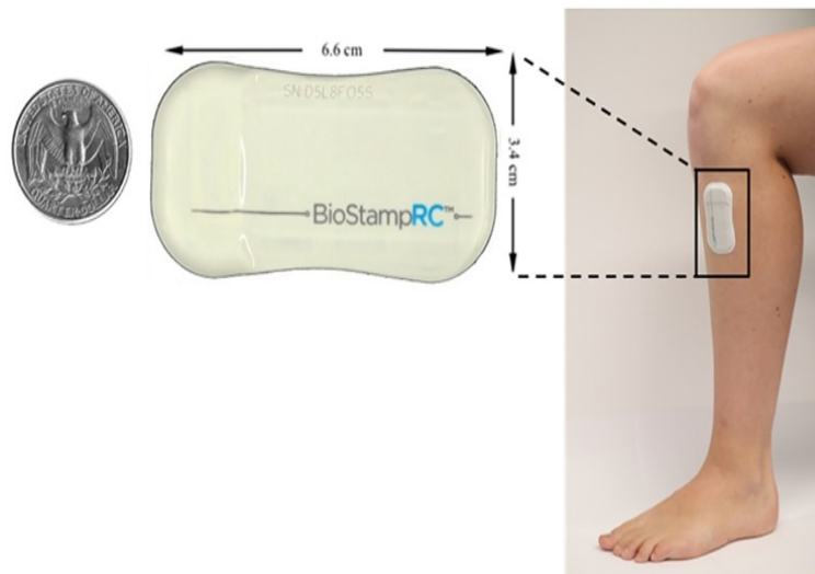
Figura 1.14: "BioStampRC a novel wireless, skin-mounted conformal inertial sensor. Figura adaptada de [Moo+17]"
