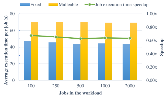
Figure 9. Average job execution time on different fixed and malleable workloads with an increasing number of jobs.
