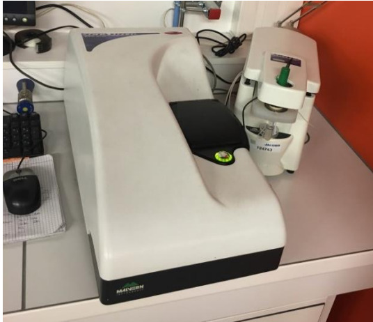
Figure 32. ZetaSizer Malvern Nano ZS used to measure the size and zeta potential
