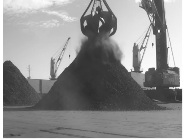
Fig. 2: Direct unloading onto the wharf with a grab.
