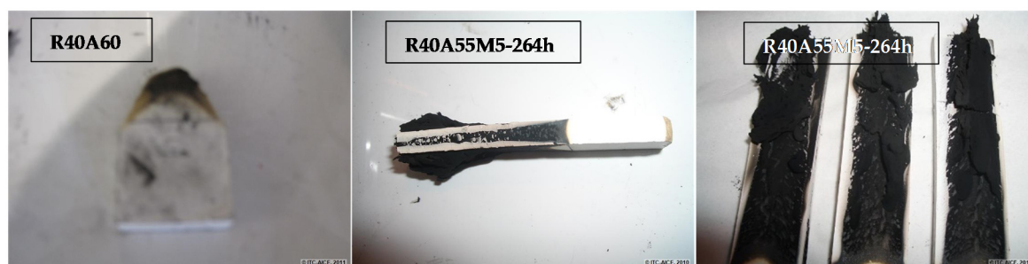
Figure 12. Combustion residues obtained from the limiting oxygen index (LOI) measurement.
