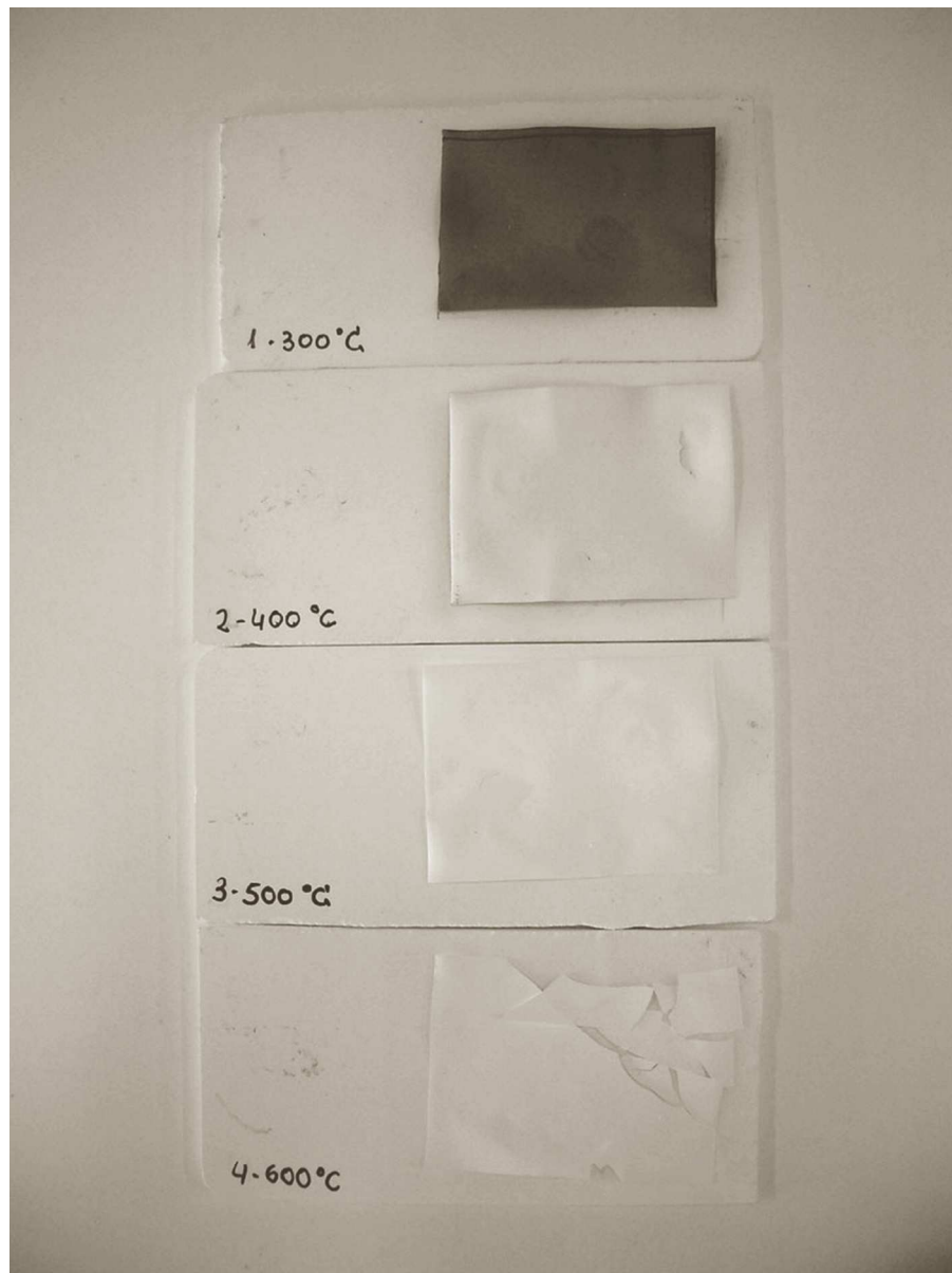
Fig. 5. Aspect of the sheets heated at 2°C/min up to different maximum temperatures.
