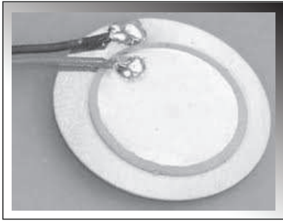
Fig. 1 Piezoelectric sensor with electrodes and electrical connection
