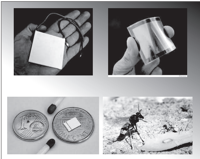
Fig. 3 Clockwise: Peltier coolers composed of thermoelements. Polymeric photovoltaic cell. A photovoltaic-like behavior has been observed in Vespa orientalis hornet. Meso Peltier cooler. Hornet taken from [77], rest from manufacturers
