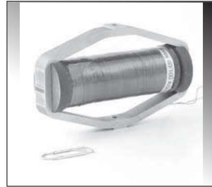
Fig. 2 Magnetostrictive actuator with surrounding coil and mechanical pre-tension
