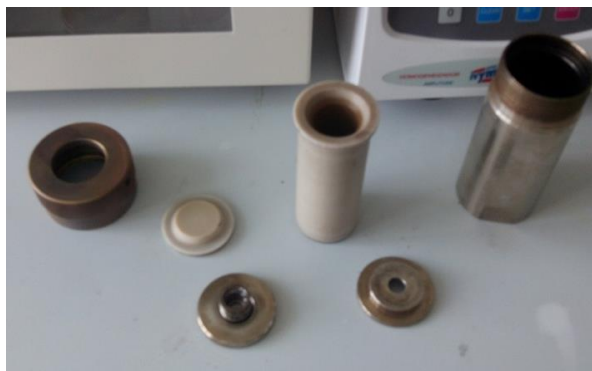
Figure 22. Solvothermal reactor used in the process.
