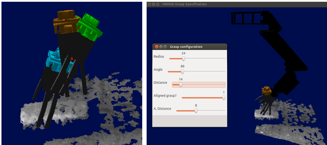
Figure 7. The interface shows the desired pose in orange, the reachable approach pose in green and the pose where the jaw will close in blue (left). It is also possible to see the full arm configuration (right).
