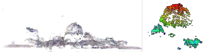
Fig. 24. laser scan of a sea urchin (left), and the camera view and user grasp specification (right). The laser stripe is detected on the image and used for the reconstruction of the 3D points..
