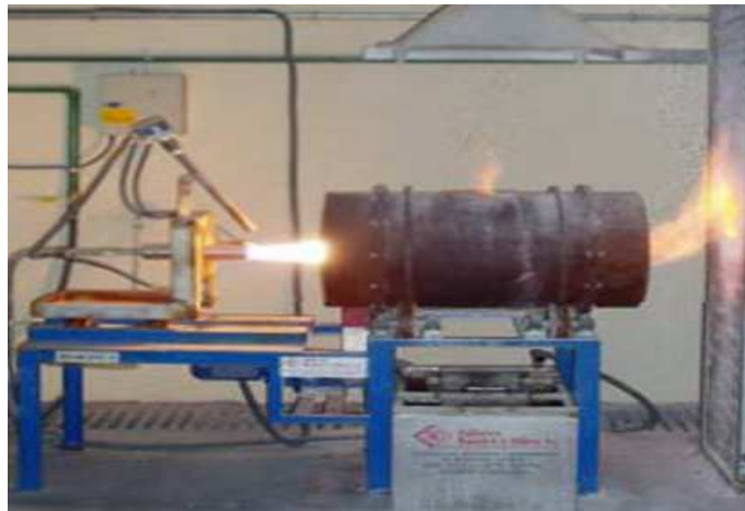
Figure 1 Rotary furnace employed to obtain the frit
