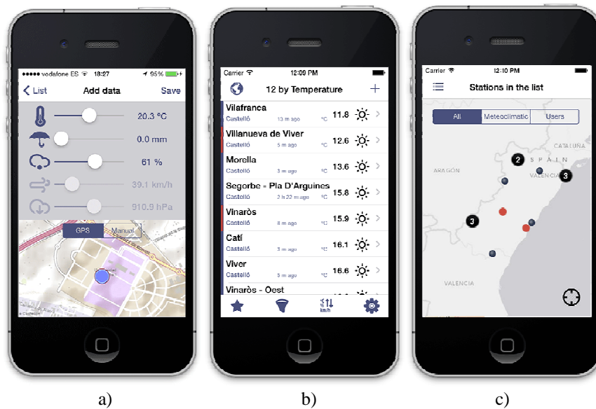
Fig. 3. From left to right, a) users are able to enrich the system at any time with climate information, b) the application shows, in different colours, information provided by direct and indirect users, red and blue, respectively. c) map shows clustering without differentiate sensors data source but particular stations.
