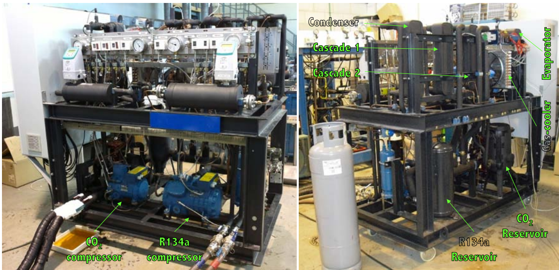
Figure 1. View of the cascade refrigeration prototype
